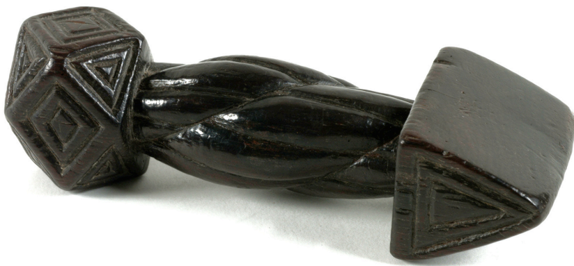
18th century sailmaker's liner, used to smooth out creases and flatten stitches in canvas sails.
