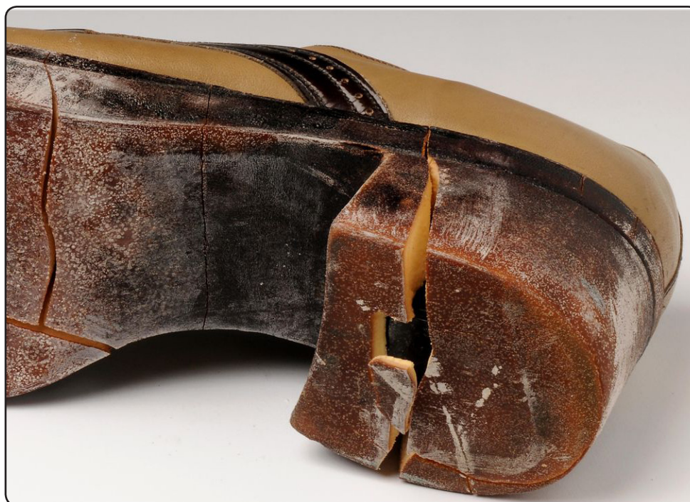
The polyurethane sole of this shoe shows cracking caused by hydrolysis – a process of deterioration which can occur in a warm, moist environment. © National Museum of Wales
