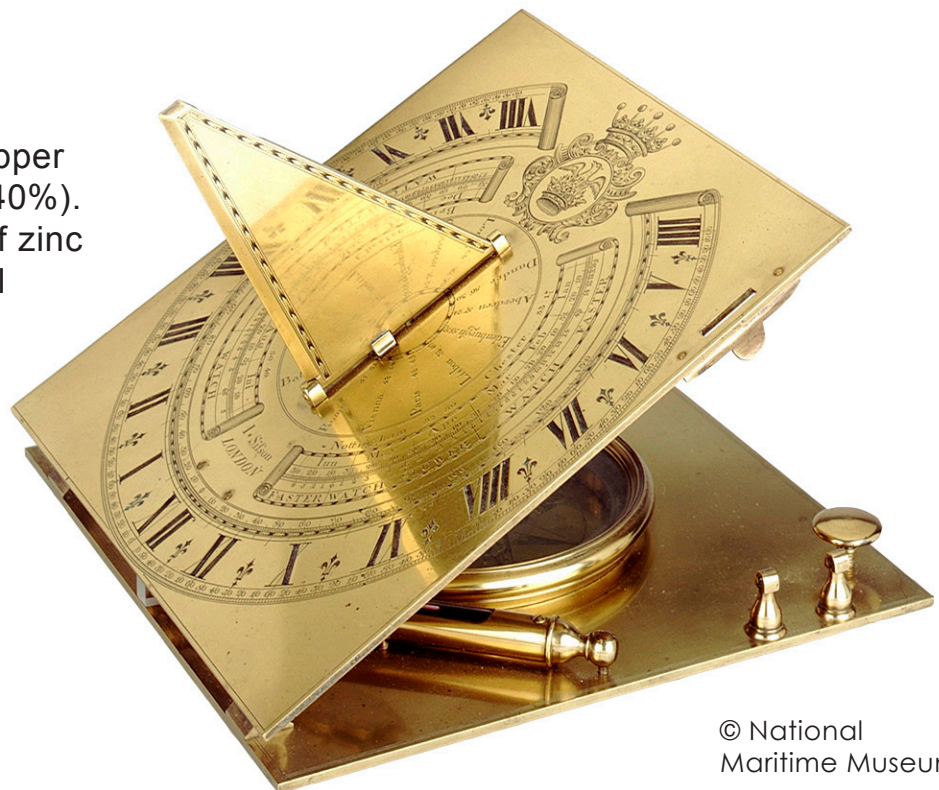
Brass inclining dial, c.1737. This square shaped dial has a brass base-plate, a compass and two brass spirit levels.
