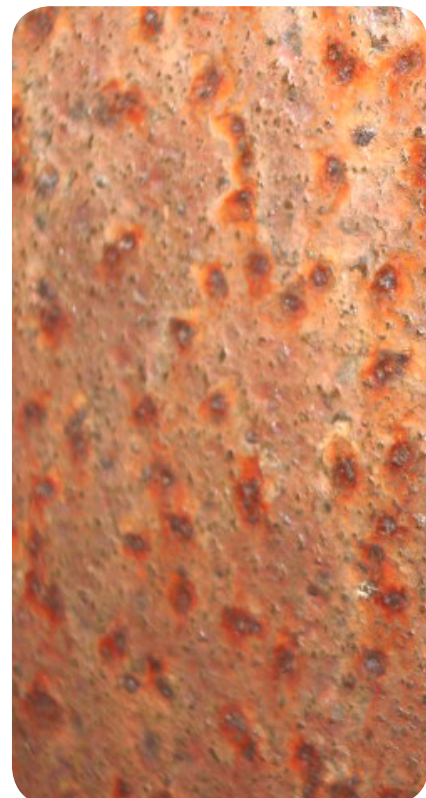
Steel corrosion on Anthony Caro's 'Dream City' (1996) in the Yorkshire Sculpture Park, showing surface pitting and blistering. © Zelda Baveystock
