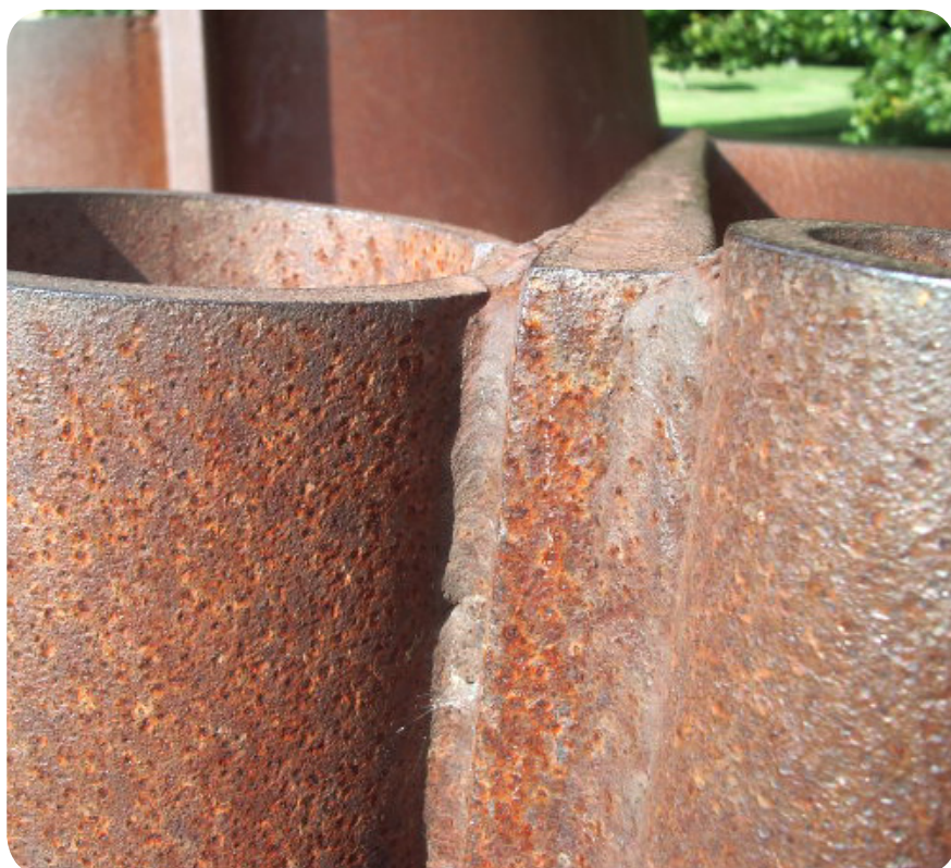
Steel corrosion on Anthony Caro's 'Dream City' (1996) in the Yorkshire Sculpture Park, showing surface pitting and blistering. © Zelda Baveystock
